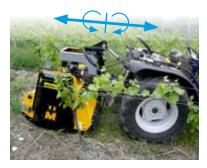
Gear box with twin freewheels enables use on tractors with different PTO stub shaft rotational directions (optional).
