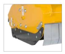
The narrow, vertical wearing skids at the sides prevent any shearing action or damage to the crop due to drifting on slopes.
