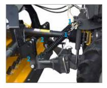
Improved steering capability and traction with front-mounted attachment thanks to the front shock-absorbing linkage springs (1) and increased lift (2) for the mulcher to cater for tractors with a low coupling height (Cat. 1+2) (optional).
