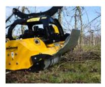
Specially shaped wearing skids and the durable material deflector plate optimise the material flow (optional).
