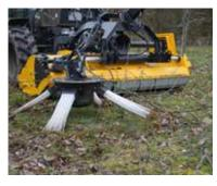
Additional hydraulic accessories such as the chopped-wood rake, cutting disc and string cutting head make the machinery suitable for many different uses (optional).
