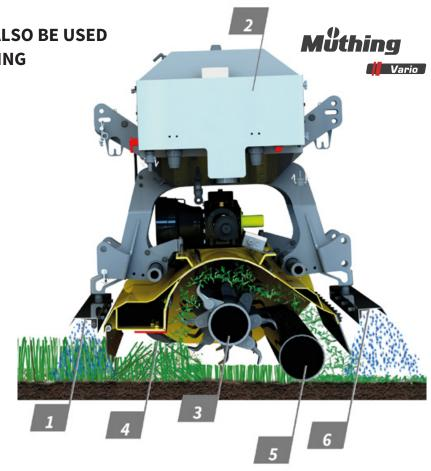
The **main components** are a spray bar (1) at the front, the tank with pump (2), the double spiral rotor (3) with shear bar (4), the support roller (5) and a spray bar (6) at the rear.
