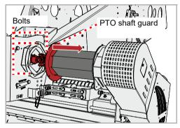
Remove the nuts from the PTO shaft guard and push the PTO shaft guard in
