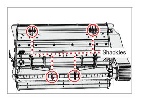
The chopper can be removed from the baler for transportation, for example on a trailer. Only use the designated points for attaching the lifting device. The machine must be securely positioned.
