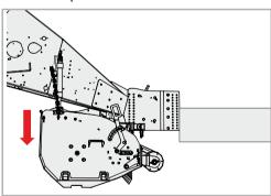
Use the tractor's control unit to lower the chopper into the work position
