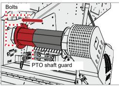
▶ Fit the PTO shaft guard and secure it with nuts
