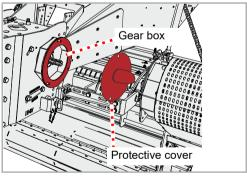
▶ Fit the protective cover to the gear box and secure it with nuts
