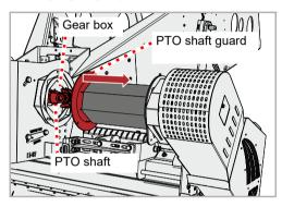
▶ Push back the PTO shaft guard and connect the chopper's PTO shaft to the gear box. Make sure that the lock pins engage securely.
