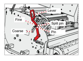
Initially set the lower shear bar to "Coarse".
