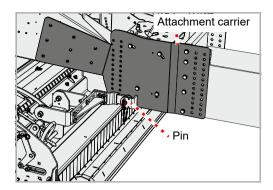
▶ Remove the pins on both sides of the attachment carrier
