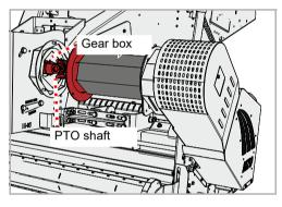
▶ Disconnect the chopper's PTO shaft from the gear box
