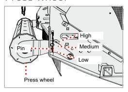
The press wheel can be adjusted depending on the height of the swath.
