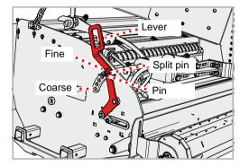
The length of the material to be chopped can be set using an upper and a lower shear bar. This setting is dependent on the characteristics of the material to be chopped. Therefore check the setting later on, when you are in the field.
