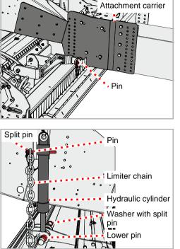
Remove the pins on both sides of the attachment carrier
