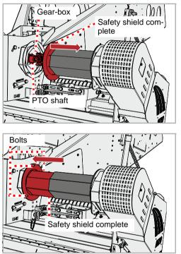
Push back the PTO shaft guard and connect the chopper's PTO shaft to the gear box. Make sure that the lock pins engage securely.
