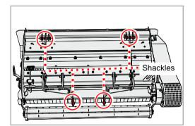
The chopper can be removed from the baler for transportation, for example on a trailer. Only use the designated points for attaching the lifting device. The machine must be securely positioned.
