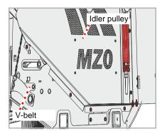
The V-belt is tensioned by an idler pulley. If the V-belt is not sufficiently tensioned, it must be retensioned. If there are any tears or the V-belt is damaged, it must be replaced.
