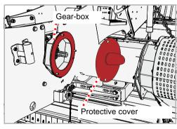
▶ Fit the protective cover to the gear box and secure it with nuts
