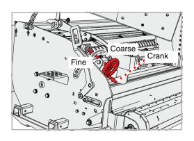
Initially set the upper shear bar to "Coarse". If you required a finer cut, adjust the upper shear bar towards "Fine".
