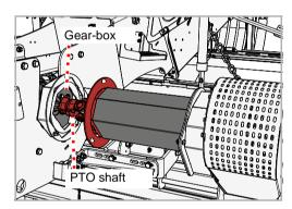
▶ Disconnect the chopper's PTO shaft from the gear box
