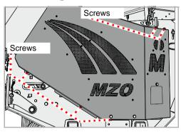
You will have to remove the safety cover for the purpose of checking.
