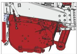
Use the tractor's control unit to lower the chopper into the work position
