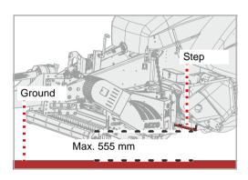
The space between the tread and the ground must not exceed 550 mm.
