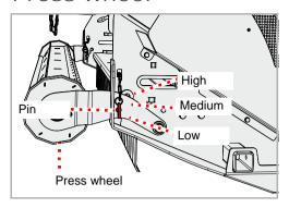
The press wheel can be adjusted depending on the height of the swath.
