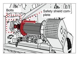
Remove the nuts from the PTO shaft guard and push the PTO shaft guard in
