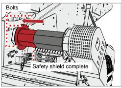
▶ Fit the PTO shaft guard and secure it with nuts
