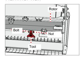
You have the option to choose between the hammer flail tool set or the shackle flail tool set. When carrying out replacement work, always replace the entire tool set.
