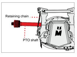
**Do not lay the attached PTO shaft in the retaining chain** The attached PTO shaft must not lie in the retaining chain. *A PTO shaft lying in the retaining chain will be damaged during road transport or when operating the lower link.*
