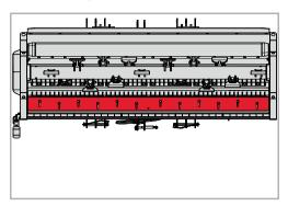
The degree of shredding can be altered using a cutting bar. You can use it to determine how finely the material should be shredded.
