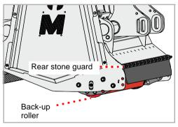
Depositing the cut material behind the support roller is the most common setting. The support roller runs directly over the ground.
