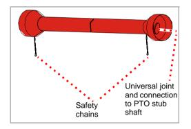
Check the PTO shaft for contamination and clean if required. Dust in conjunction with oil and grease results in increased wear
