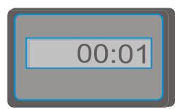
An electronic operating hours counter displays the actual operating duration. This means that data can be recorded precisely and used, for example, for calculations. Faults can often be eliminated quickly and easily. In the event of hydraulic problems, first check:
