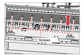
After adjusting the cutting bar you must check whether any tools are touching the cutting bar.
