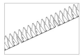
The short chopping bar optimises the material feed. This produces better cutting.
