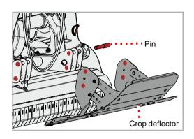
Insert crop deflector plate and fix in place with four pins
