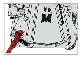
If you are using a crop deflector plate, side support legs are needed. The use of side support legs is also recommended for front attachment of the machine.
