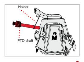
**Do not lay the attached PTO shaft in the holder** The attached PTO shaft must not lie in the holder. *A PTO shaft lying in the holder will be damaged during road transport or when operating the lower link.*
