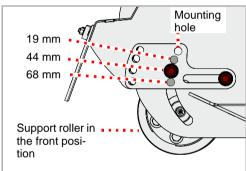
Without rakes, the support roller can be in the front or rear position.
