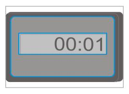
An electronic operating hours counter displays the actual operating duration. This means that data can be recorded precisely and used, for example, for calculations. Faults can often be eliminated quickly and easily. In the event of hydraulic problems, first check:
