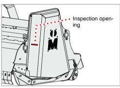
The V-belt is tensioned by a clamping plate. If the V-belt is not sufficiently tensioned, it must be retensioned. If there are any tears or the V-belt is damaged, it must be replaced.
