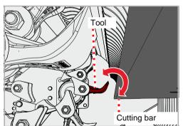
Check whether any of the tools are touching the cutting bar.
