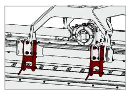
If the clearance height is not sufficient, a lower link extension is available for the sliding headstock and sliding dual headstock.
