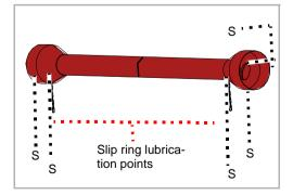
In case of heavy usage or in extreme operating conditions, such as a very dusty environment, more frequent lubrication is required.
