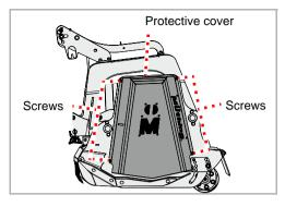
Remove the screws, remove the protective cover
