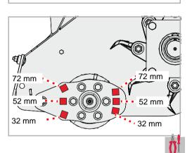
> Select the corresponding hole pattern for the desired working depth
