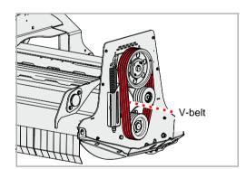
The V-belt unit consists of four narrow V-belts.
