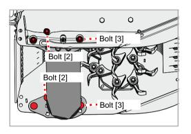
Also loosen and remove bolts [2] and [3] on the opposite side of the housing
