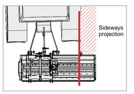
The machine may be mounted behind or in front of the tractor either directly or offset to one side.
