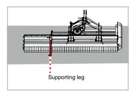
Check that the machine is securely positioned. The support leg has been lowered and the machine housing is on the ground.
