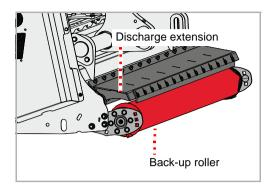
Depositing the cut material in front of the support roller is only possible with a discharge extension [+]. The support roller runs over the cut material.
