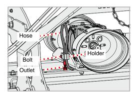
The gear box is equipped with a hose for draining the oil.
