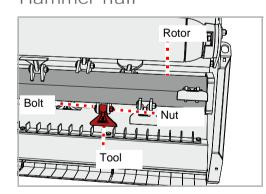
You have the option to choose between the hammer flail tool set or the shackle flail tool set. When carrying out replacement work, always replace the entire tool set.
