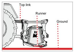
Adjust the top link so that the runners are parallel to the ground
