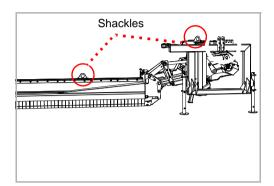
For transport on, for example, a trailer, the machine can be raised. Only use the designated points for attaching the lifting device. The machine must be securely positioned.
