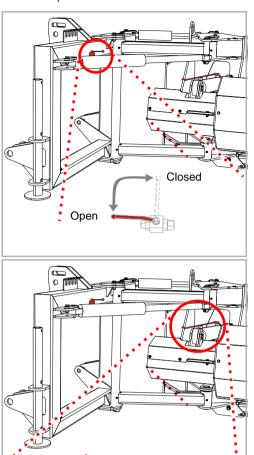
▶ Set the stop valve to "Open" position on hydraulic cylinder 1
