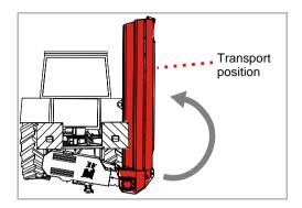
Using the tractor's control device, fold the machine into the transport position
