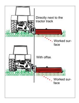
▶ Using the tractor's control device, swivel out the machine as required
