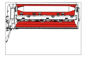
A metal insert protects the housing from wear.
