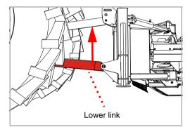
Position the lower link over the three-point power lift of the tractor at a height which will enable the machine to be high enough for transport
