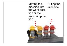
Connecting the hydraulic hoses to one double-acting control valve each
