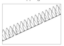
A second counter-cutter makes work easier if the material to be mulched in the field is very long. They guide the material towards the tools, thereby making better cutting possible.
