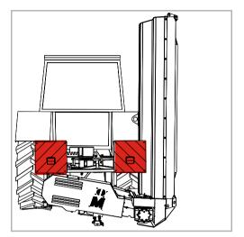
For transporting the machine on the road, warning signs with integrated lighting equipment are available.
