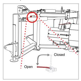
▶ Set the stop valve to "Open" position on hydraulic cylinder 1
