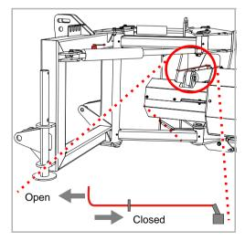
▶ Set the stop valve to "Open" position on hydraulic cylinder 2
