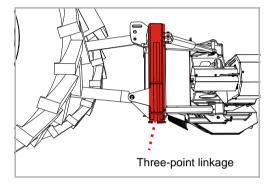
▶ Adjust the top link so that the three-point stand is vertical
