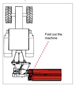
Using the tractor's control device, fold out the machine into the work position
