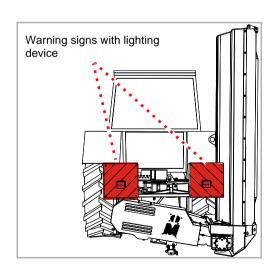
▶ Check lighting device for correct function
