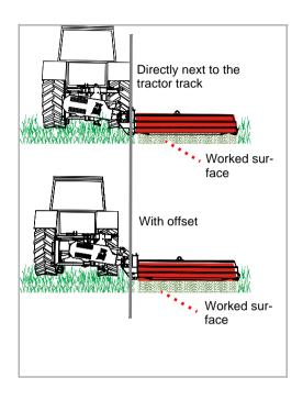
▶ Using the tractor's control device, swivel out the machine as required
