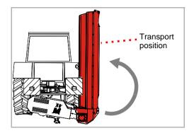
Using the tractor's control device, fold the machine into the transport position
