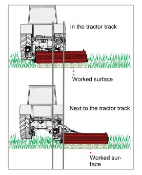
Do not swivel out when the machine is lowered.
