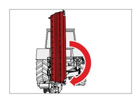
Using the tractor's control device, fold out the machine into the work position
