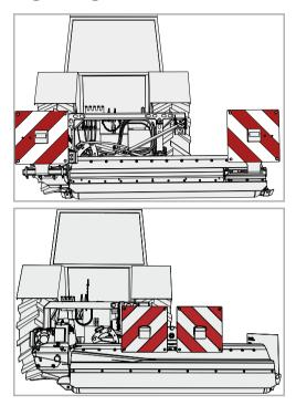
For transporting the machine on the road, warning signs with integrated lighting equipment are available.
