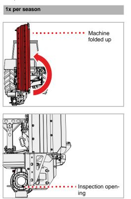
> Fold the machine up using the control device on the tractor
