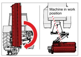
Using the tractor's control device, fold out the machine into the work position
