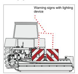
Check lighting device for correct function
