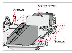
Remove the screws, remove the safety cover.
