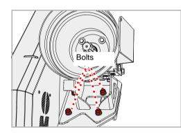
Loosen the lock nuts.
