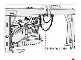
**Do not lay the attached PTO shaft in the retaining chain** The attached PTO shaft must not lay on the retaining chain. *A PTO shaft laying on the retaining chain will be damaged during road transport or when operating the lower link.*
