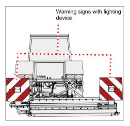
Check lighting device for correct function
