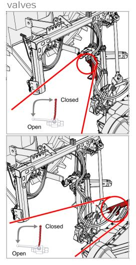
Set the stop valve to "Closed" position on hydraulic cylinder 1
