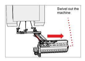
• Using the tractor's control device, swivel out the machine as required
