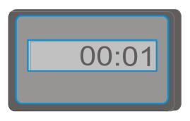
An electronic operating hours counter displays the actual operating duration. This means that data can be recorded precisely and used, for example, for calculations.
