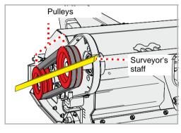
▶ Check the alignment of the drive belts. Use a surveyor's staff or similar. The gauge must lie flat on both pulleys and be in alignment.
