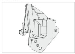
Imlement triangle for front mounting with carrier vehicles:
