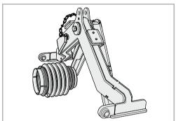
The coupling triangle can only be used for machines with mechanical drive.
