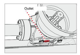
▶ Place a collection container under the outlet for the waste oil
