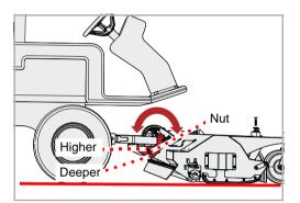
Adjust the machine so that the runners are parallel to the ground.
