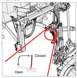
Set the stop valve to "Closed" position on hydraulic cylinder 1
