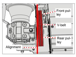
▶ Check the alignment of the pulleys. The rear pulley must be in line with the front pulley.
