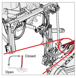
▶ Set the stop valve to "Open" position on hydraulic cylinder 2
