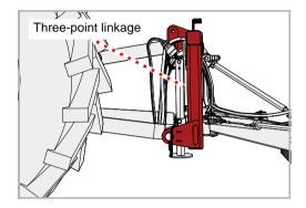
▶ Adjust the top link so that the three-point stand is vertical
