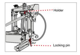
The locking pin must be removed for mulching.
