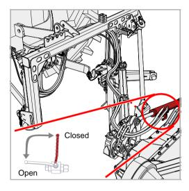
▶ Set the stop valve to "Closed" position on hydraulic cylinder 2 The machine is now safely set down.
