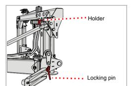
▶ Check that the machine is secured with the locking pin
