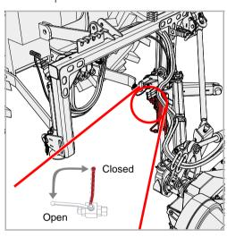
▶ Set the stop valve to "Open" position on hydraulic cylinder 1
