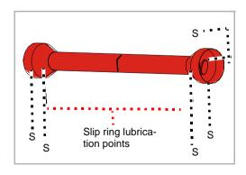
In case of heavy usage or in extreme operating conditions, such as a very dusty environment, more frequent lubrication is required.
