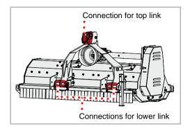
The linkage can be mounted on category I or category II tractors with connections for lower link balls.
