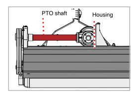
▶ Check whether the PTO shaft is parallel to the housing
