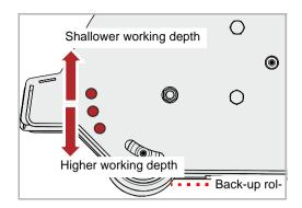
▶ Raise or lower the machine so that it is at the desired working depth
