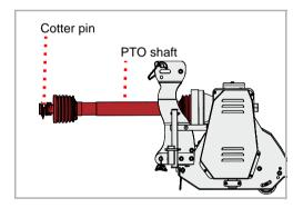
▶ Connect the PTO shaft to the PTO stub shaft of the tractor and ensure that the cotter pin is locked in place on the PTO shaft
