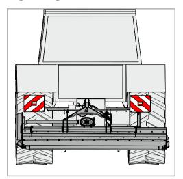
For transporting the machine on the road, warning signs with integrated lighting equipment are available.
