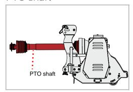
▶ Disconnect the PTO shaft from the tractor
