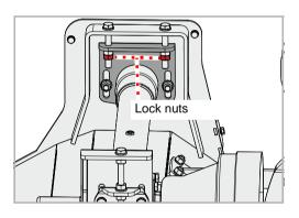
▶ Loosen the lock nuts.
