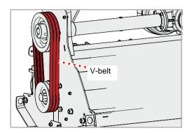
The drive belt unit consists of three narrow drive belts.
