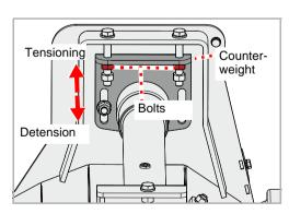
▶ Slacken the drive belts using the nut
