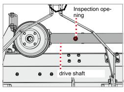
▶ Loosen the screw on the inspection opening with an Allan key and remove the screw
