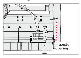
are any tears or the V-belt is damaged, it must be replaced.
