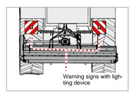
▶ Check lighting device for correct function
