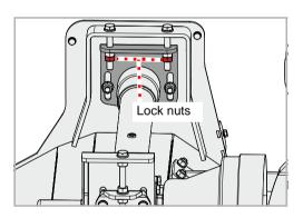
▶ Loosen the lock nuts.
