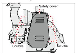
▶ Remove the screws, remove the safety cover.
