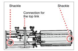
For transport on, for example, a trailer, the machine can be raised. Only use the designated points for attaching the lifting device. The machine must be safely parked in the working position.
