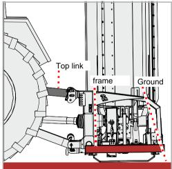
Adjust the top link so that the frame is parallel to the ground
