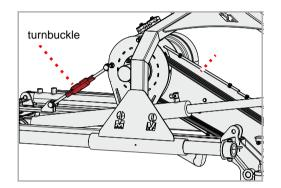
Release the drive belt tension with the help of the turnbuckle
