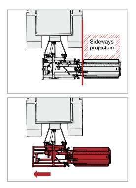
The machine can be transported in working position or in transport position.
