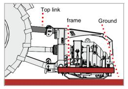
Adjust the top link so that the frame is parallel to the ground
