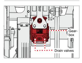
The outlet valve is located under the gearbox.
