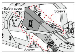
Remove the screws, remove the safety cover.
