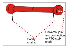
▶ Check presence and correct function of safety chains If the safety chains are not present or are heavily worn:
