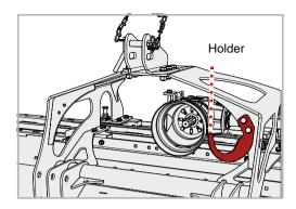
▶ Disconnect the PTO shaft from the tractor and secure with the holder
