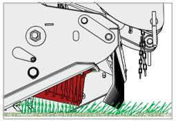
Suction is generated via the short-cut flap, pulling the short-cut grass upright and optimising the appearance of the lawn.
