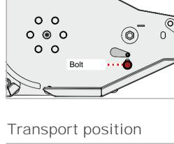
Insert the bolt in the bottom hole on both sides of the machine and retighten them
