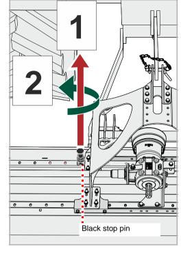
▶ Pull up the black stop pin and turn it through 90°. The stop pin is locked in the upper position.
