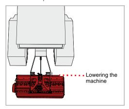
Using the tractor's control device, lower the machine into the work position
