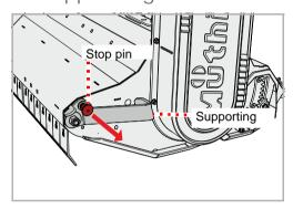
▶ Pull out the stop pin and screw tight
