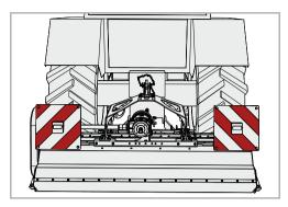
For transporting the machine on the road, warning signs with integrated lighting equipment are available.
