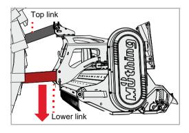
▶ Lower the lower link until the top link is no longer under compressive or tensile strain
