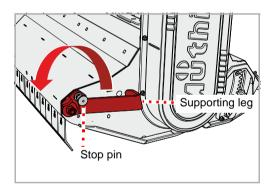
Swing the support leg downwards and secure in the bottom position with the stop pin
