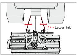
Adjust the lower link so that the machine has little play to the left or right
