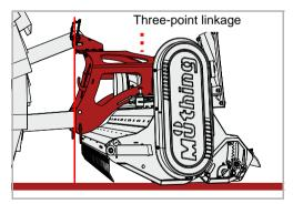
▶ Adjust the top link such that the 3-point trestle is vertical with respect to the ground
