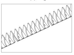
The short chopping bar optimises the material feed. This produces better cutting.
