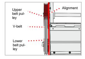
▶ Check the alignment of the belt pulleys. The upper belt pulley must be in line with the lower belt pulley.
