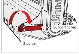
▶ Swing the support leg upwards and secure in the top position with the stop pin
