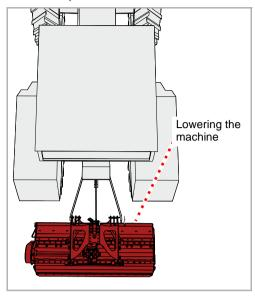
▶ Lower the machine to its work position
