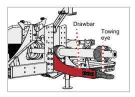
The drawbar with shackle must be adjusted in height to the coupling of the tractor. Have the adjustment carried out by a specialist workshop.
