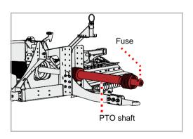
▶ Connect the PTO shaft to the tractor's PTO stub shaft and ensure that the retainer is locked in place on the PTO shaft
