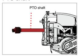
Disconnect the PTO shaft from the tractor
