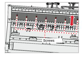
You can alter the degree of shredding using a cutting bar.
