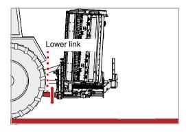
Adjust the height of the lower links via the three-point linkage system of the tractor
