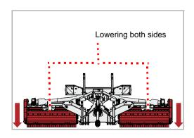
Lowering is carried out via the corresponding control valves on the tractor.
