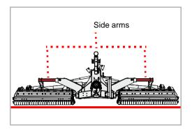
The side arms of the machine should be parallel to the ground.
