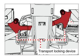
The machine is folded out into the work position via the corresponding control valves on the tractor.
