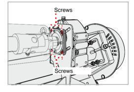
▶ Undo the bolts on the gear box but do not remove them
