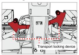
Unlock the transport locking devices using the control unit on the tractor
