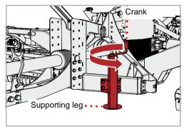
Move the supporting leg into the lower position using the crank
