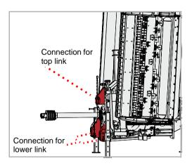
The linkage can be mounted on category I or category II tractors with connections for lower link balls.
