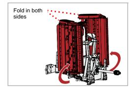
▶ Fold the machine in using the control valve of the tractor. Make sure that the two transport locking devices lock into place securely.
