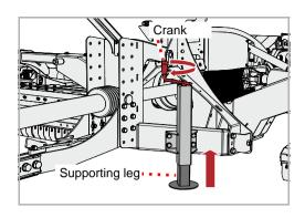
▶ Move the supporting leg into the top position using the crank. The supporting leg is fixed in the top position.
