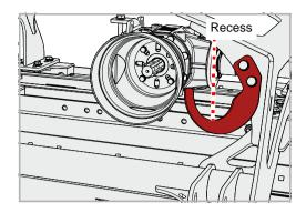
▶ Raise the PTO shaft slightly and take it out of its stowage system
