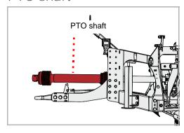
▶ Disconnect the PTO shaft from the tractor
