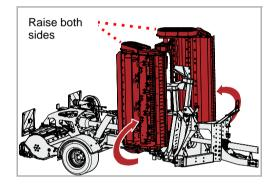
▶ Fold the machine in using the control valve of the tractor. Make sure that the two transport locking devices lock into place securely.
