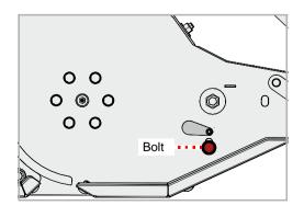
Insert the bolt in the bottom hole on both sides of the machine and retighten them
