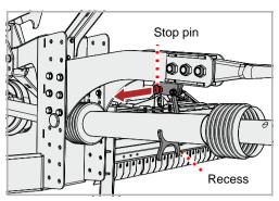
The PTO shaft hangs in the stowage system.
