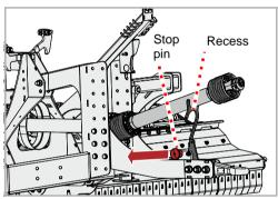
▶ Fold in stowage system and allow locking bolt to engage
