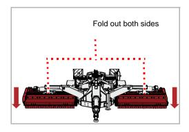
▶ Fold out both sides of the machine using the control unit on the tractor
