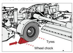
Secure the machine against rolling away using the wheel chocks.
