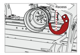
▶ Lift PTO shaft and place in stowage system
