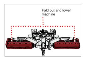
▶ Fold out machine and lower into the work position
