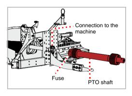
The PTO shaft and drawbar have been adjusted to fit your tractor by your dealer. The drawbar is positioned above or below the PTO shaft.
