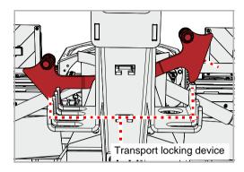
To fold the machine in, both transport locking devices of the machine must be unpressurised.
