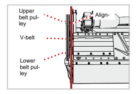
▶ Check the alignment of the belt pulleys. The upper belt pulley must be in line with the lower belt pulley.
