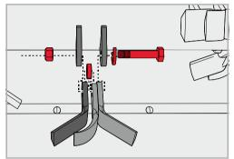
Y blades require less power during work. When using a Y blade set, the rotor must be replaced at a specialist workshop. It is not possible to assemble the Y blades on a standard rotor.
