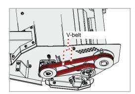
The V-belt unit consists of two narrow V-belts.
