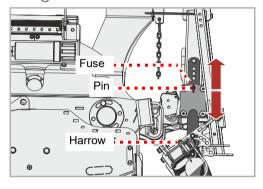
The height can be adjusted in 25 mm increments.
