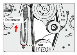
▶ Slacken the drive belts using the nut
