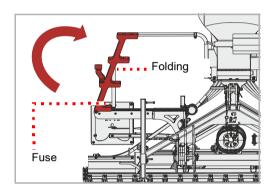
When travelling on roads or uneven surfaces, the folding ladder must be secured.
