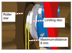
▶ Measure the gap between the last roller star and the limiting disc
