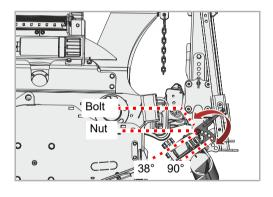
The working angle can be set between 38° and 90° in 13° increments.
