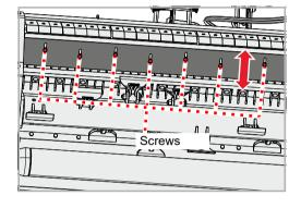
After adjusting the cutting bar you must check whether any tools are touching the cutting bar.
