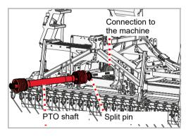
Generally, the PTO shaft is already connected to the machine. If the PTO shaft is replaced or after maintenance work to the PTO shaft, it will be necessary to connect it to the machine.
