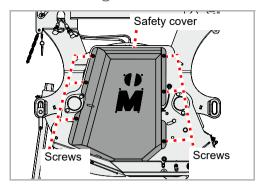
▶ Remove the screws, remove the safety cover.
