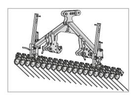
The harrow aligns the mulch. This enables the next mulcher to spread and process the mulch uniformly.
