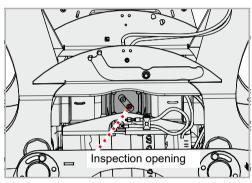
▶ Loosen the screw on the inspection opening with an Allen key and remove the screw
