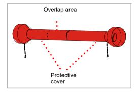
▶ Check the PTO shaft for contamination and clean if required. Dust in conjunction with oil and grease results in increased wear
