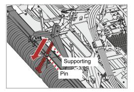
The pressure roller can be removed and set down separately from the machine.
