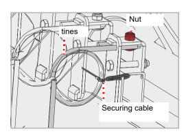
The tines wear faster or slower depending on the field conditions and frequency of use. Wear can be managed by adjusting the height.
