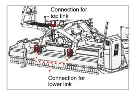
The attachment can be mounted on category III tractors with connections for lower links.
