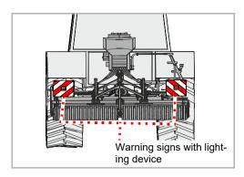
▶ Check lighting device for correct function
