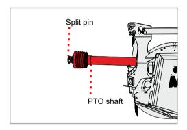
Connect the PTO shaft to the PTO stub shaft of the tractor and ensure that the cotter pin is locked in place on the PTO shaft
