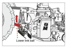
▶ Position the lower link over the three-point power lift of the tractor at a height which will enable the machine to be high enough for transport
