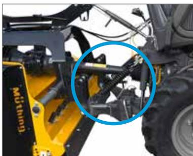
Improved steering capability and traction with front-mounted attachment thanks to the front shock-absorbing linkage springs (optional).
