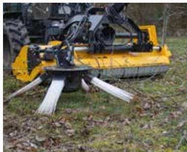
Additional hydraulic accessories such as the chopped-wood rake, cutting disc and string cutting head make the machinery suitable for many different uses (optional).
