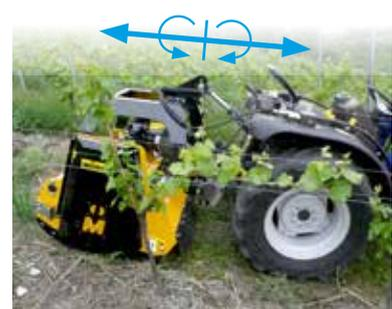
Gear box with twin freewheels enables use on tractors with different PTO stub shaft rotational directions (optional).
