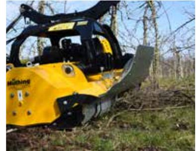
Specially shaped wearing skirts and the durable material deflector plate optimise the material flow (optional).
