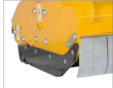
The narrow, vertical wearing skirts at the sides prevent any shearing action or damage to the crop due to drifting on slopes.
