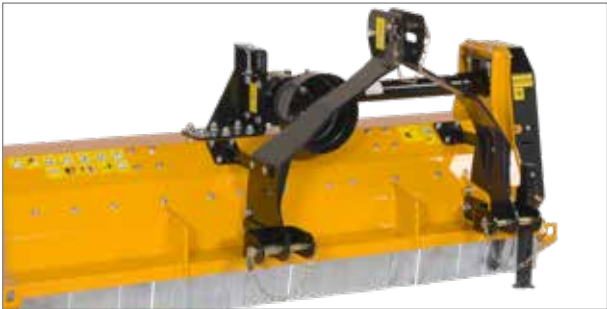
The headstock of the MU-ECOTOP can be unscrewed and moved behind the tractor and offset to the side.
