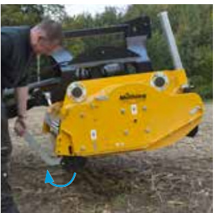
Easy adjustment of the swivelling support roller, even without an assistant.
