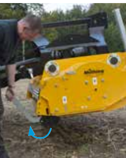
Easy adjustment of the swivelling support roller, even without an assistant.
