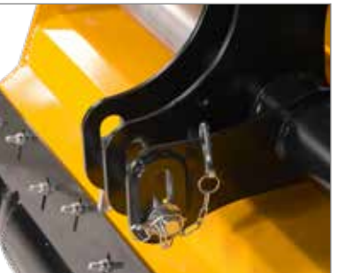
Elongated holes on the upper and lower link mounting points ensure excellent ground following in combination with the swivelling support roller.
