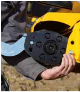
The scraper keeps the support roller clean and reduces dust development (optional).
