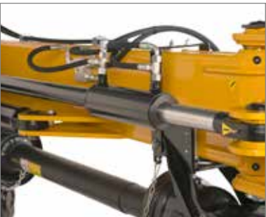
In the event of a problem, the hydraulic non-stop collision protection device swivels the flail mower out of the collision zone effectively.
