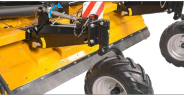
The turnbuckle allows you to quickly set the correct cutting height.
