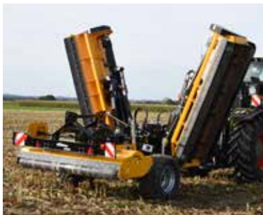
Folds in and out quickly to achieve a transport width of less than 3 m.
