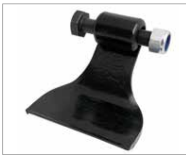
Indestructible: Made out of rolled steel and weighing 2.7 kg, the MU-Farmer® hammer flails ensure a long service life even under high throughput of plant mass or with light ground contact.
