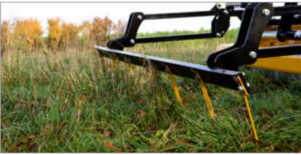
Insect rescuer: A specially designed, hydraulically folding bracket with integrated angled tines frightens away insects and small organisms from the front of the flail mower and causes them to flee. (optional for working widths of 1.6 m and 2.20 m)
