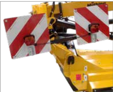
Warning signs with lighting equipment and lighting beam with sturdy mounting wand without moving parts
