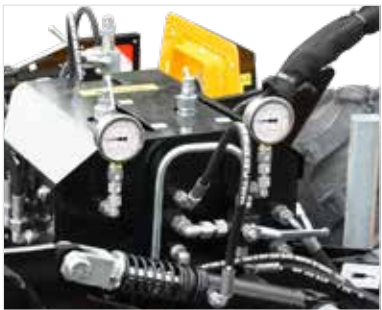
Tidy: The on-board hydraulics with the hydro-pneumatic MU-SOFA® weight transfer system.
