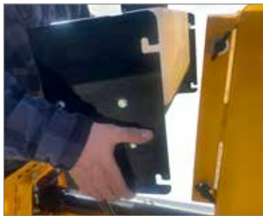
Pump unit can be removed for maintenance purposes and to protect against frost.
