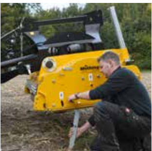
Easy adjustment of the swivelling support roller, even without an assistant.
