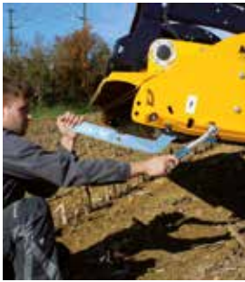
Easy adjustment of the swivelling support roller, even without an assistant.
