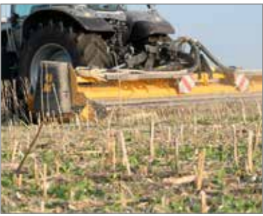
Solo use of the flail mower is possible through easy removal of the seeder.
