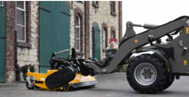
Vehicle-specific mounting parts: The low coupling point ensures a good overview thanks to the low linkage position. Good accessibility to the hydraulic connections.
