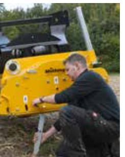
Easy adjustment of the swivelling support roller, even without an assistant.
