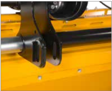
Elongated holes in Cat. 2 on the upper and lower link mounting points ensure excellent ground adaptation in combination with the swivelling support roller.
