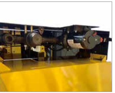
Pump unit consisting of intake filter, electric pump, pressure filter and pressure regulating valve.
