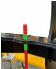
The correct work position can be determined conveniently using a height indicator visible from the cab.
