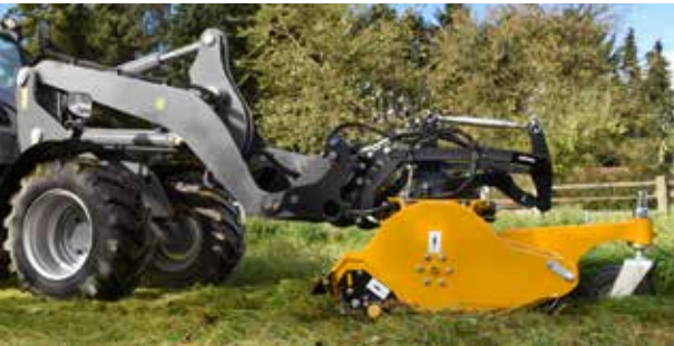
Virtual pulling point - A MÜthing patent: The flail mower is pulled with low rolling resistance instead of pushed and thus follows every ground contour perfectly.
