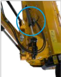
Secure transport lock for on-road driving or when transporting the tractor/equipment combination on a passenger car trailer.
