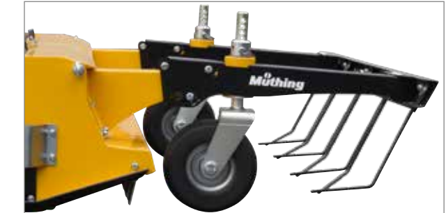
Front support wheels installed as standard facilitate handling and improve ground following. They are vertically adjustable and swivel through 360°. A forward-mounted insect rescuer is available optionally.
