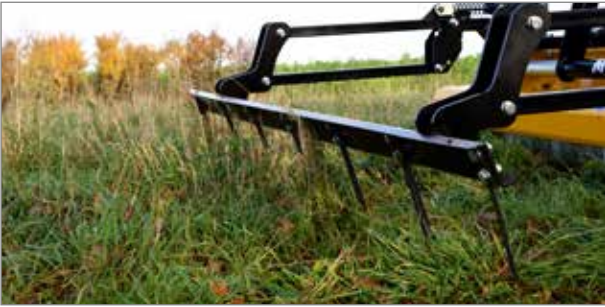
Insect rescuer: A specially designed, hydraulically folding bracket with integrated angled tines frightens away insects and small organisms from the front of the flail mower and causes them to flee. (optional for working widths of 1.6 m and 2.20 m)
