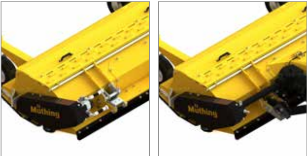
Both mechanical and hydraulic drive are possible, optimised for the vehicle.
