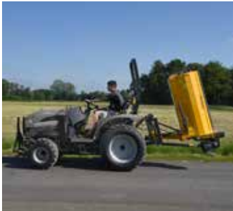
Secure transport lock for on-road driving or when transporting the tractor/equipment combination on a passenger car trailer.
