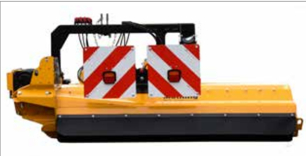
Rotating warning signs with LED lighting equipment and lighting equipment support, with sturdy mounting and without moving parts
