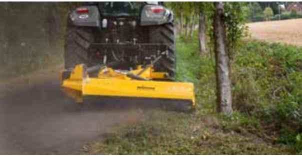
A large adjustment range makes it possible to work both behind and alongside the tractor. Narrow access tracks and side strips can be mulched just as easily.
