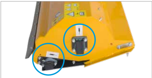
Easily accessible bearing points for quick maintenance.
